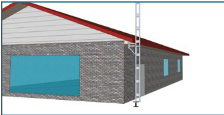
STEP 2 PLACE BASE OF POST OVER A SCREW JACK AND LEAN AGAINST THE ROOF EDGE OF THE BUILDING. REPEAT AND SPACE NO MORE THAN 4m TO DESIRED LENGTH
