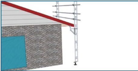
STEP 5 USING A LADDER, PLACE THE ALUMINIUM TUBE RAILS IN POSITION, THEN TIGHTEN EACH COUPLER
